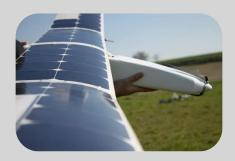
Integration on wings of drone for increasing of fly time
